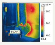
The additional heat in the 'after' pictures is due to smaller, uninsulated components. Adding insulation would decrease thermal losses even further.
