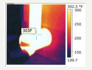
The installation of thermal boiler covers has reduced the thermal losses from temperatures exceeding 300F down to around 100F or below, depending on room temperature.
